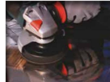
Pre-polish with a soft backing pad and hard polishing fleece in combination with white polishing paste. Start off slow and then build the speed up as the paste warms and works itself into the metal.
