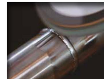
On a slow to medium speed setting use the angle grinder with the Metabo VKS wheel to remove the weld tarnish. The VKS wheel will gently remove the tarnish and any light scratches, but it will not drastically effect the weld profile, if anything a smoothing result will be obtained.
