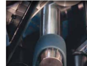
With a burnishing machine and a nylon web fleece belt you can remove minor scratches and achieve a smooth satin like finish in one easy step. Use on half speed, setting 3\*.
