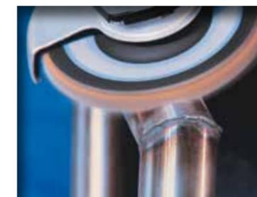
Using the KLS wheel you can remove the weld and achieve a high quality surface finish in just one step. Due to the tough yet flexible nature of the KLS wheel you can work with the form of the pipe profile. Select speed setting 3\* and work in the direction of the pipe.
