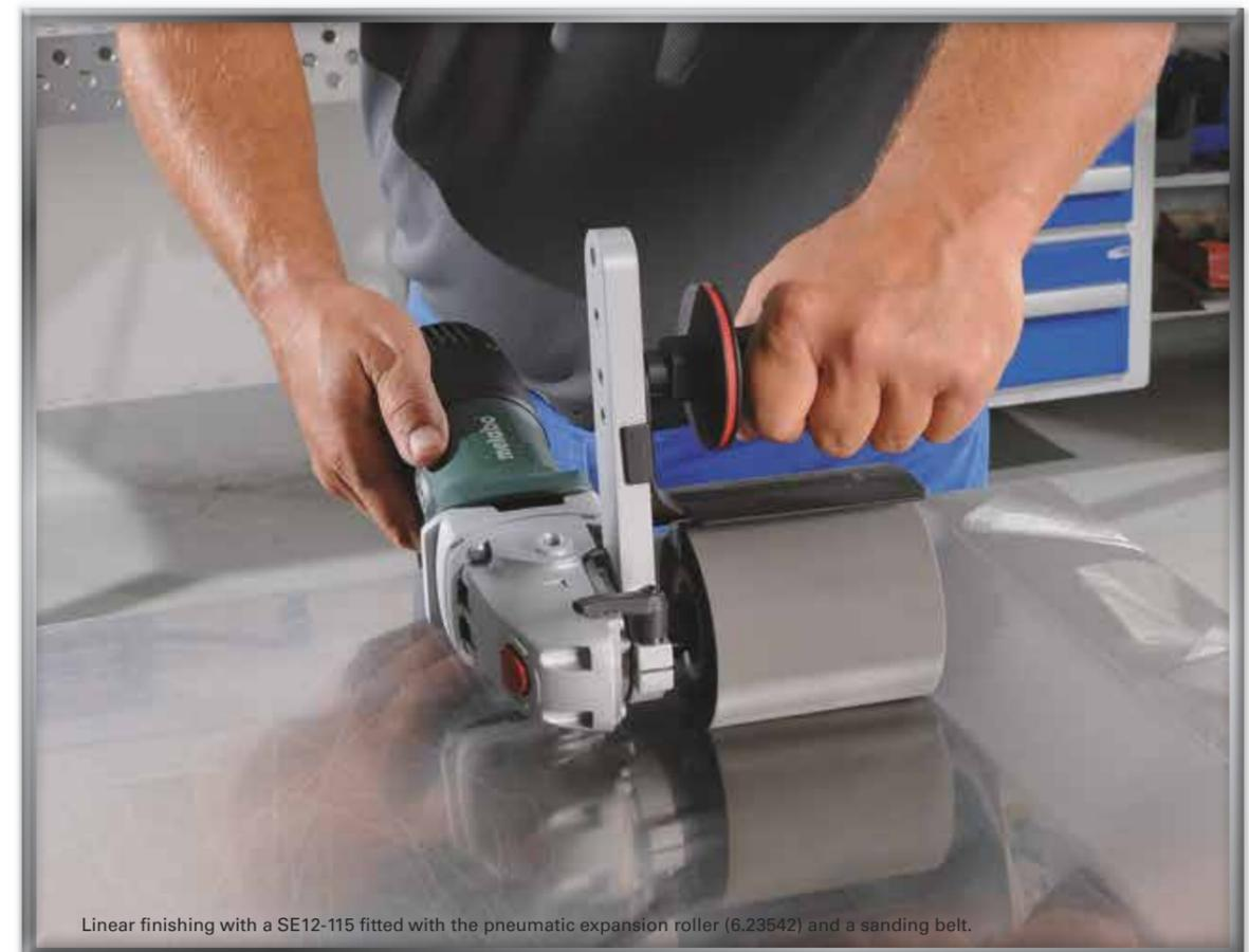
Linear finishing with a SE12-115 fitted with the pneumatic expansion roller (6.23542) and a sanding belt.
