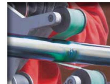
Use either the corded or cordless RB machines with the ceramic grain P 80 grit sanding paper to remove the weld in one step. The ceramic grain paper offers high material removal rates together with extremely long life. Select high speed setting 6\* and remove a TIG weld seam in seconds.
