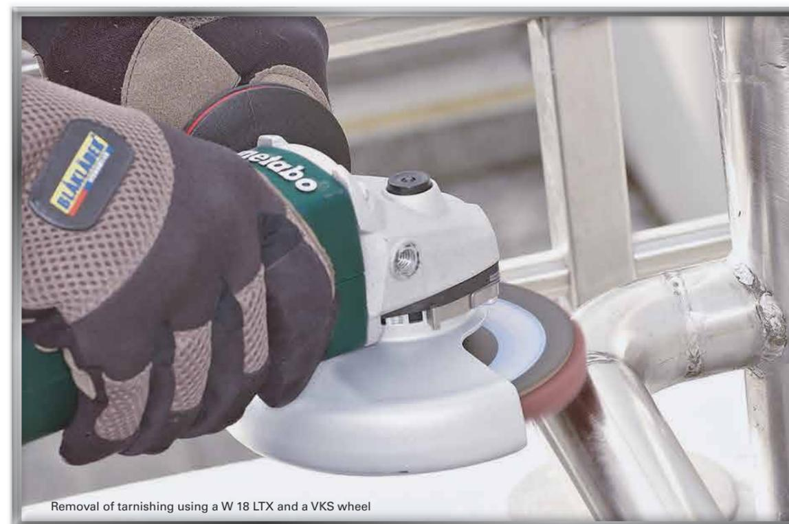
Removal of tarnishing using a W 18 LTX and a VKS wheel
