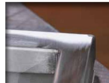
After the weld seam has been removed burnish one side of the box section using the P 60 wheel in a linear motion. If so required be careful to not round the edges.
