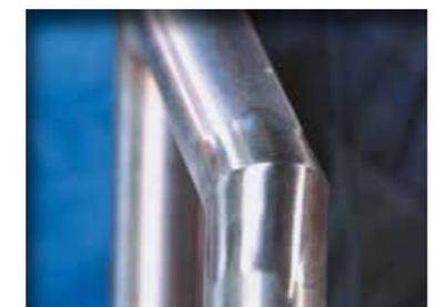
A perfect corner angle is formed and neighbouring surfaces are not damaged. The image shows a clean and precise result. Slight rotation marks may be left around the weld area. These can be later removed with one of the RB pipe belt sanders.
