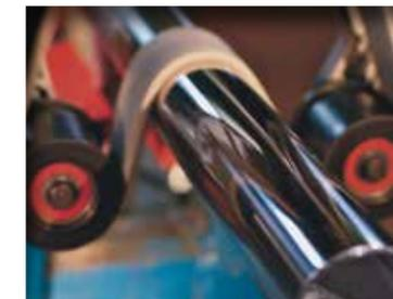
Using the white felt belt, a low rpm and the white polishing paste evenly work over the surface. For a really high gloss finish clean with talc and a cloth, change belts and repeat the process using polishing paste blue. Increase the belt speed after the paste warms into the metal.
