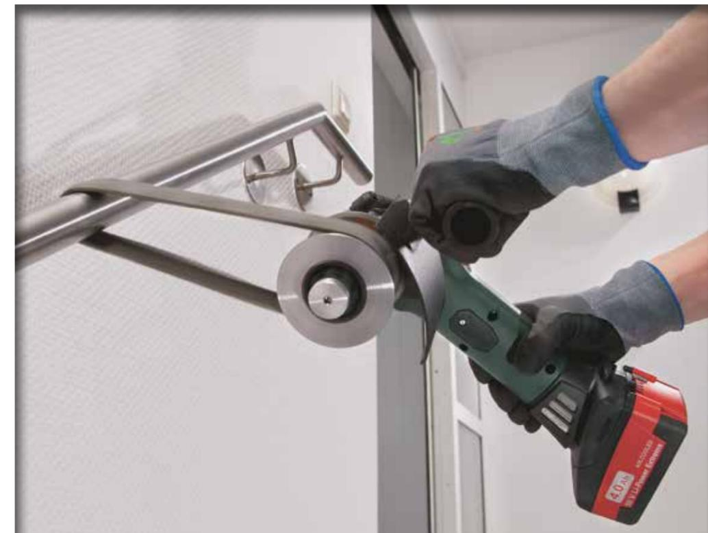
For closed off rail sections close to a wall the Metabo belt drum and "buttonhole" belt accessory option will prove particularly useful, especially if the rail is closed off with wall brackets on either side of your working area. With the buttonhole belts you can then loop & close the belt behind the rail. With this method you will achieve a perfect uniform result 360o around the handrail. Going mobile? Go cordless with the S 18 LTX 115.
