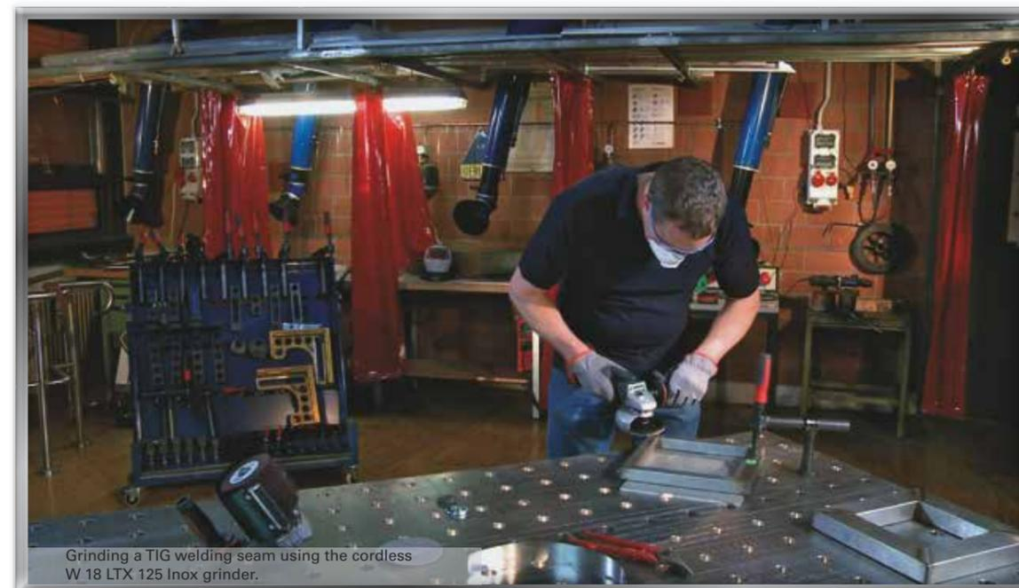
Grinding a TIG welding seam using the cordless W 18 LTX 125 Inox grinder.
