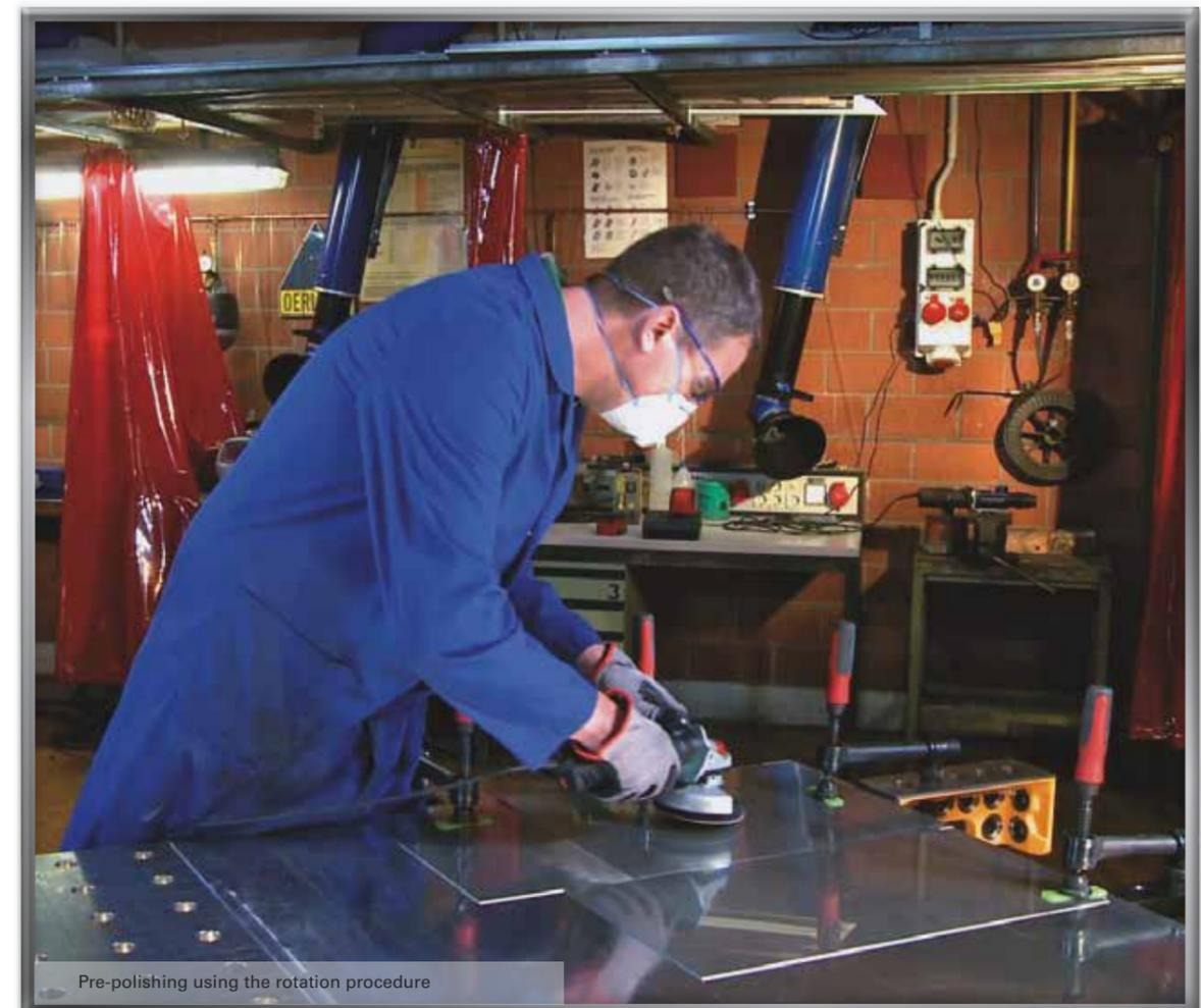
Pre-polishing using the rotation procedure
